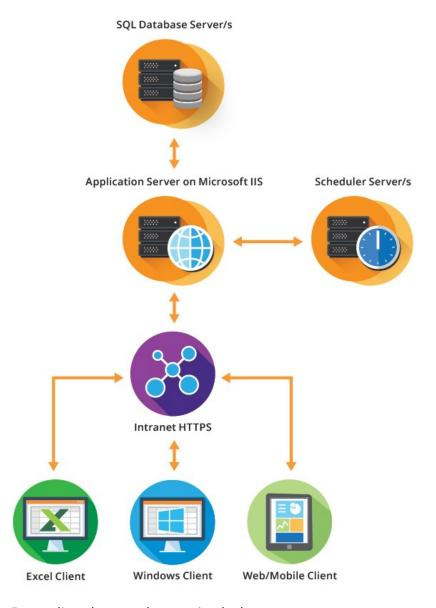
For medium, large, and enterprise deployments, server components must be hosted on separate servers for optimal performance. Additionally, for larger deployments, we recommend multiple Scheduler servers.
